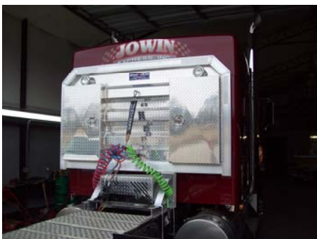
Photo 2 – Most firms hang them on the siderails but Jowin Express found the perfect place to install the Arctic BREEZE unit – right under the headache rack.
